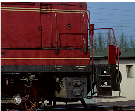
The first three series of V60 (left) were equipped with rectangular coal fired Dofa oven for keeping cooling water on temperature. Later series had a rounded oil oven (right).
